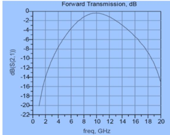
Fig 4 Response of the Schottky Diode
